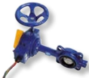
Wafer butterfly valve CE with reducer and switch. Valve to be used between flanges. Ductile cast iron casting, inox lenses.
