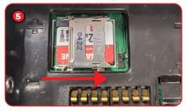
INSERT THE SD CARD CORRECTLY AND SLIDE THE HOUSING UNTIL IT 'CLICKS'.
