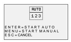
Pressing the key (ENTER) the process that automatically performs 3 consecutive analyzes at intervals of 120 "and calculates the average, starts. Pressing the key (**MENU**) the procedure making 3 consecutive analyzes and calculating the average, acquiring the single analysis data while pressing the
