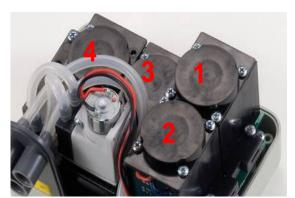
It is also possible to replace the pump or even the analysis chamber, thus avoiding in case of need to return the instrument to the manufacturer or the distributor.
